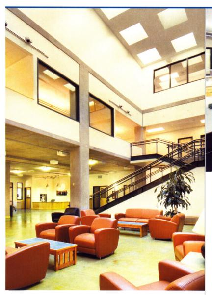
"We have a 3-story atrium space in the center of the building to provide natural daylighting to the exhibit area and all the surrounding spaces on each floor. The atrium has a monumental open stair connecting the main entry of the building with the second floor."
